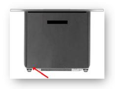
Figure 2.1 Microsoft Surface Side View showing AC/Main rocker switch
